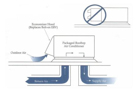
Note: Greenheck ERV control centers have separate contacts for exhaust fan, supply fan and wheel motors. During economizer operation, the ERV receives an economizer "make" signal from the rooftop unit and shuts down the supply fan and wheel. The exhaust fan continues to operate.
