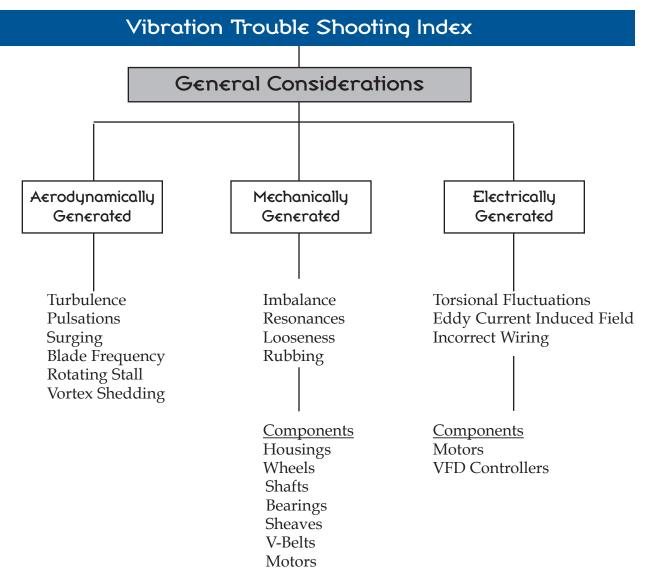
There are many different sources of vibration. One of the most difficult tasks in troubleshooting fans and systems is the systematic identification of vibration characteristics (amplitude, frequency, location, direction, units of measurement) as a function of operating point location on the fan curve and control settings. Identification of the source can be extremely difficult, in some cases requiring the services of a professional troubleshooter.
