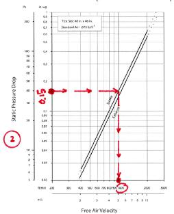
Model ESD-435 resistance to airflow (pressure drop) varies depending on louver application (air intake or air exhaust). Free area velocities (shown) are higher than average velocity through the overall louver size. See louver selection information.
